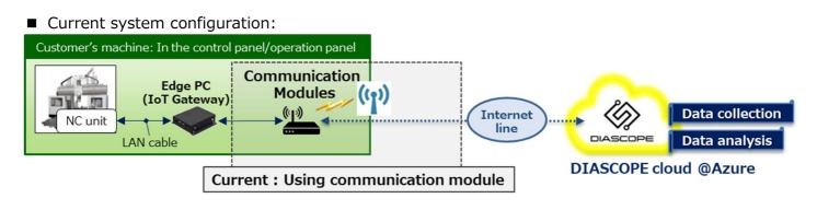
System configuration when using a commercially available mobile router:
